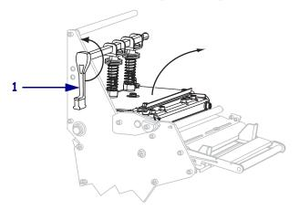
**5.** Loosen the thumb screw (not visible from this angle) that is located on the bottom of the outer media guide (1).
